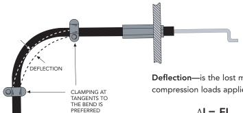
**Deflection**—is the lost motion from elastic strain resulting from tension or compression loads applied to the control. It can be calculated as follows:
